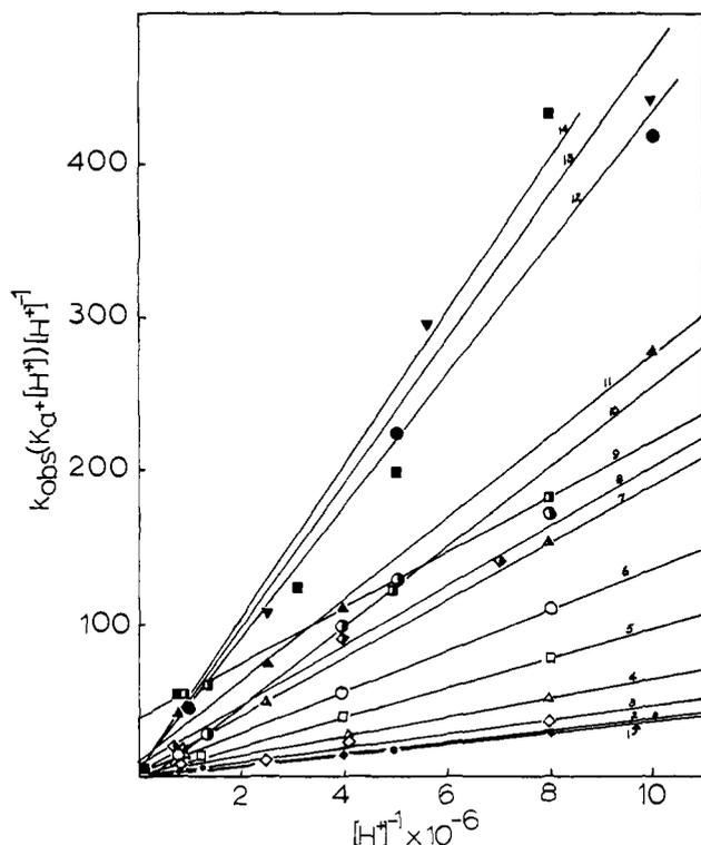
Figure 1.  $k_{\text{obs}}(K_a + [\text{H}^+])[\text{H}^+]^{-1}$  as a function of  $[\text{H}^+]^{-1} \times 10^{-6}$  for the reaction of  $\text{Ni}^{2+}$  with the following ligands: picic, ●, 1; lys, ◆, 2; gly, ◇, 3; orn, △, 4; asp, □, 5;  $\text{aspNH}_2$ , ○, 6; en, ▲, 7; dab, ◇, 8; amp, ■, 9; ga, ○, 10; digly, ▲, 11; trigly, ●, 12; tetragly, ▼, 13; IDA, ■, 14.
